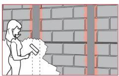
After epoxy has cured for at least two days, you can paint the wall with any standard high-quality wall paint. But first lightly sand the carbon fiber strap removing the gloss. Paint will not adhere to a glossy surface.
