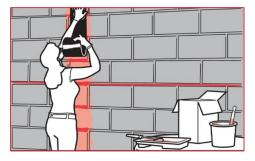
Roll strip of carbon fiber and then begin by attaching top edge at the top of the epoxied area and press into place as you unroll it all the way to the floor.
