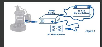
In the absence of electricity, pump sentry will convert power from a deep cycle marine battery(ies) to operate a sump pump. Under typical duty cycle conditions, using a single BCI group size 27 battery, such operation can be maintained for approximately 20 hours. To obtain even more back up time larger batteries or multiple battery banks can be configured (see Figure 2 for multiple battery parallel configuration). Back up time is directly proportional to battery capacity.
