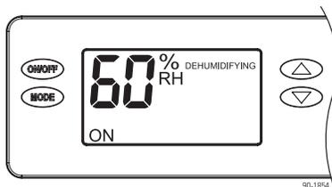
If the humidity of the air is higher than the setting, the compressor turns on and the control will display DEHUMIDIFYING, along with the measured humidity on the control screen.
