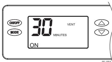
If you need to change the amount of time to operate ventilation, press the MODE button twice to display the ventilation time setting. Use the UP or DOWN button to adjust the number of minutes per hour (0–60, set to zero to turn it off) that ventilation is to run. The control will return to the dehumidifier setting display automatically.
