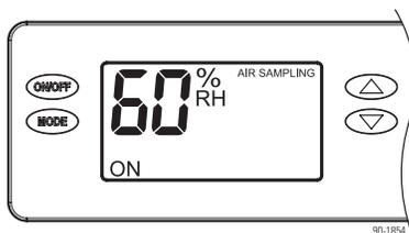
When the dehumidifier turns on, the blower circulates the air for 3 minutes before measuring the humidity level of the air. The on-board control will display AIR SAMPLING, along with the measured humidity on the control screen.
